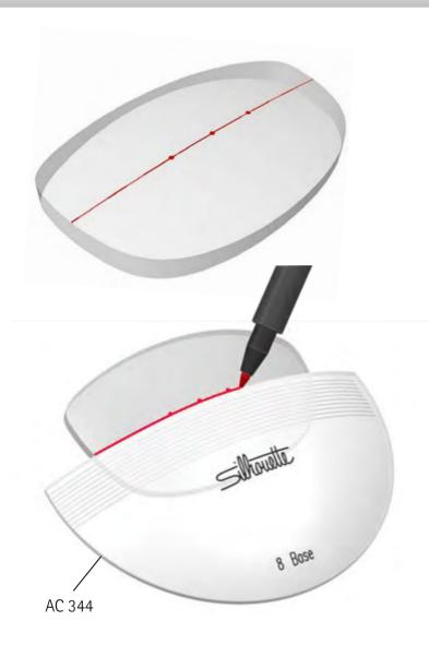
• Measure lenses in the focimeter. Mark the central axis with a waterproof pen.
