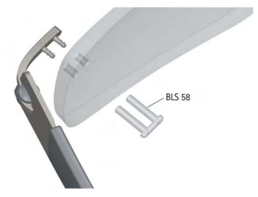
We recommend to glaze principally <u>all</u> metal frames with the harder plastic sleeves BLS 58, especially all models with stiffer temples. Due to the material characteristics and the different construction these sleeves can absorb considerably more tension. This means that the lens fixation holds multiplicatively better.
