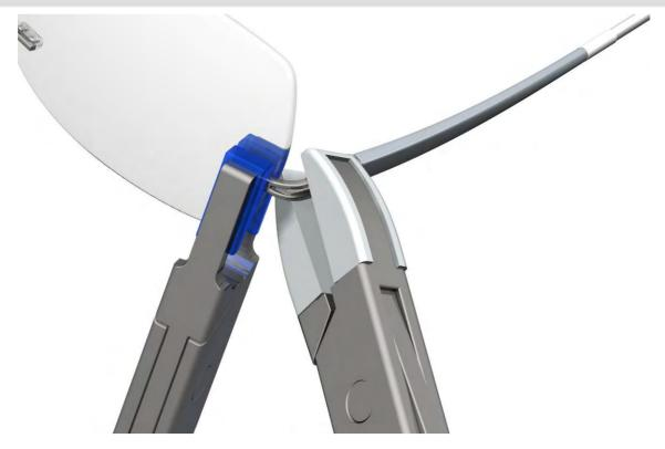
**Hold** sideparts **very firmly** in the area of the lens fixation with the universal mounting pliers. Inclinate sideparts with flat pliers.
