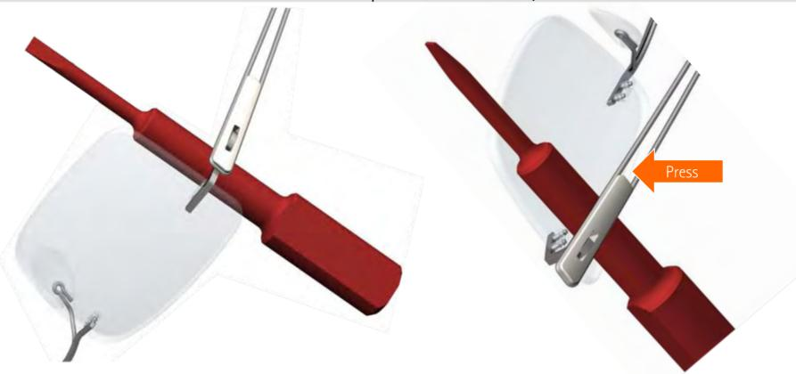
1. Place disassembly tool AC 336 to the stopping point where the trim and temple meet. Select necessary diameter, depending on distance between temple and lens. Close temple and press it through behind the rounded part.
